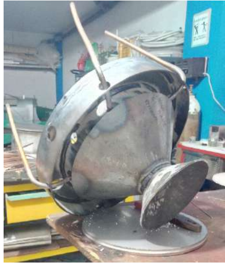
Heart of gasifier
